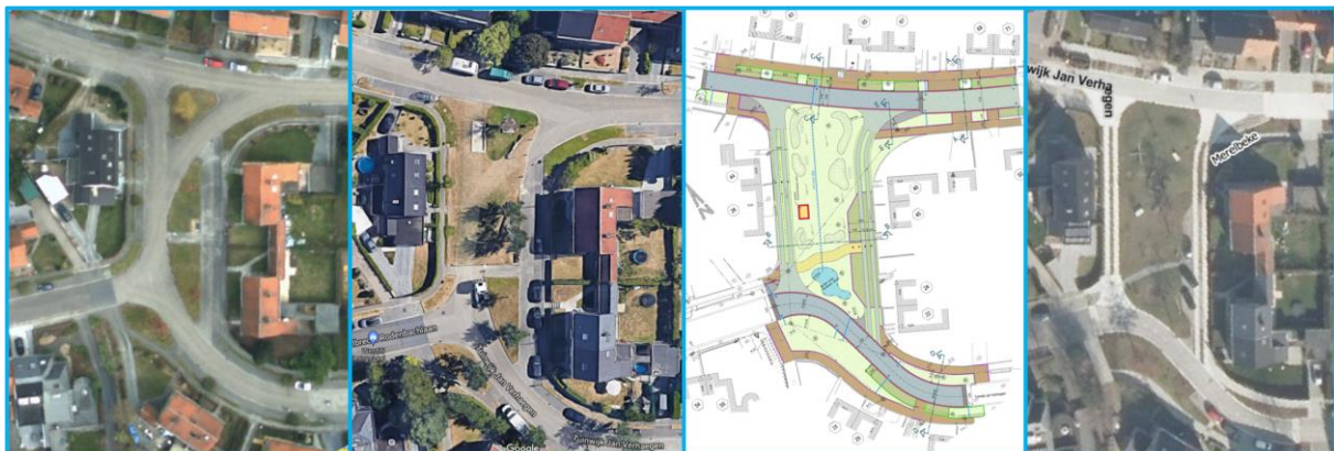
Figure 1: Leftmost: original situation of central connecting roads. Left-centre: temporary “test” installation. Centre right: final design. Rightmost: aerial photo after completion construction works, before finalising planting.
